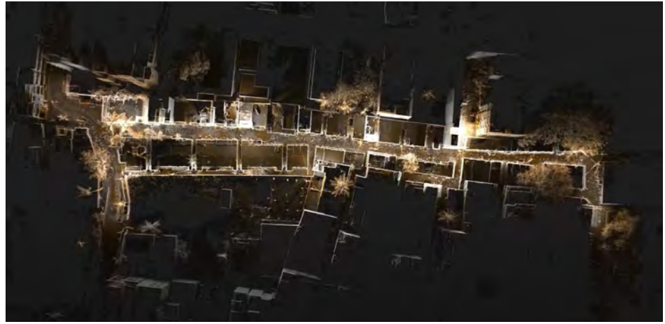
Scanning informal settlements. Photo credit: GeoSLAM
