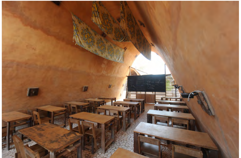
The school's classrooms are slightly sloped towards the blackboard to allow the students at the back to see properly. Credit and Copyright: © Aga Khan Trust for Culture / Amir Anoushfar (photographer)
